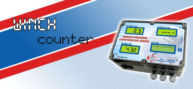
The Winch Counter is a device designed to assist the technician operating the winch. It indicates the cable's lenght when that one is unwinded and the moving speed. Also, it is optionally possible to display the depth of an instrument attached to the cable's end according to the data from another device.
