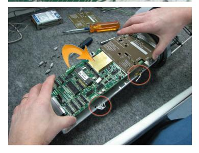
11. Reconnect the wires and the flat cable at their respective place and put back the screws
