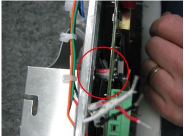
6. Use a X-acto knife to remove the glue drop at each extremity of the Compact Flash
