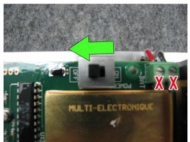
3. Disconnect the flat cable and wires on the bottom part of the board (see picture)
