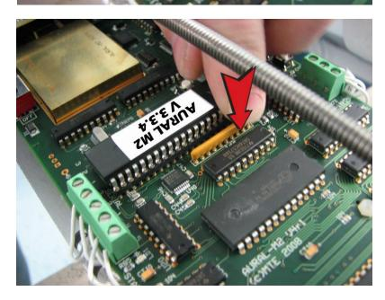
7. Apply a small pressure to enter the pins in the holes
