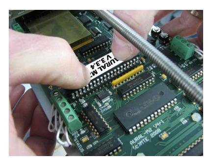
8. Inspect each pins to make sure it is well installed
