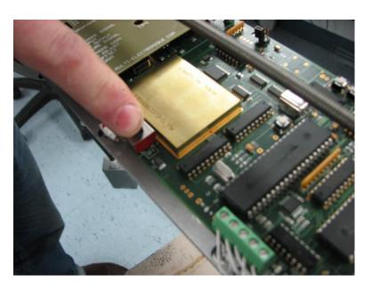
4. Use a flat screwdriver to pull out the MCU from both extremity a bit at a time
