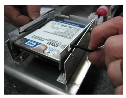
4. Remove the Hard Drive and unplug the flat cable
