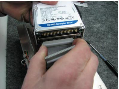
28. Use the o-ring to reinstall the Hard Drives in place
