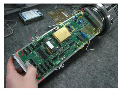
16. Be careful not to damage the temperature sensor under the board
