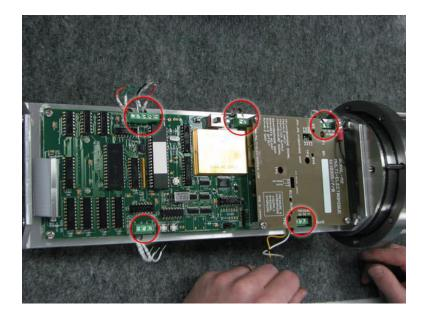
13. Use Phillips screwdriver to remove the shield
