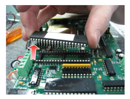
31. Insert the new MCU in place. Be sure each pin is fit in each hole
