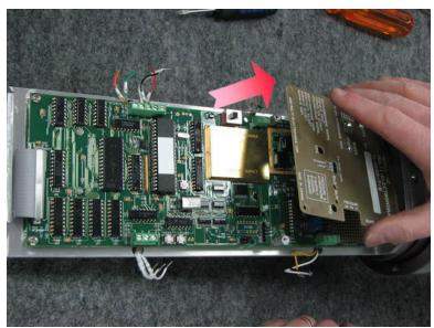
15. Use a Phillips screwdriver or a ½ box tool to remove the PCB
