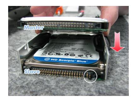
11. Use the top screws to fix the Hard Drive
