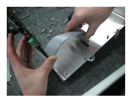
19. Disconnect the flat cable on the other side of the board
