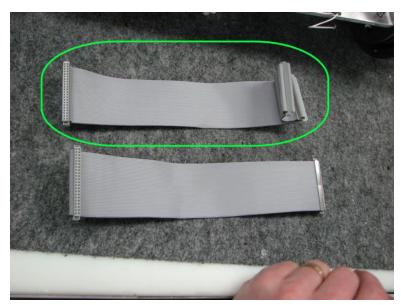
21. Plug the new flat cable using the single connector end
